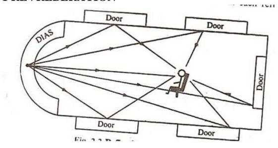
When a sound pulse is generated in a hall, the sound wave travels towards all directionand are reflected back by the walls, floors, doors, windows ceiling etc as shown in the figure.
