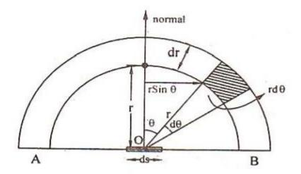
Let us consider a small element 'ds' on a plane wall AB. Assume that the element ds receive the sound energy 'E'.
